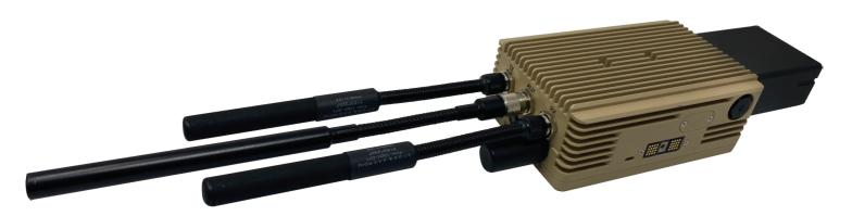
Ninja Dismount enables wearable/handheld, 360° C-sUAS protection against most commercial small Unmanned Aircraft Systems (sUAS). Ninja Dismount is a small Size, Weight, and Power (SWaP) protocol-based Radio Frequency C-sUAS system that uses sophisticated signal processing and advanced computing to defeat adversarial drones.
